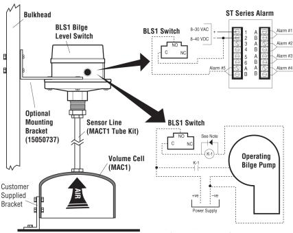
NOTE: Contact rating should be approprite for horse power of the pump. Install flyback diode across K-1 relay or DC power is used.
