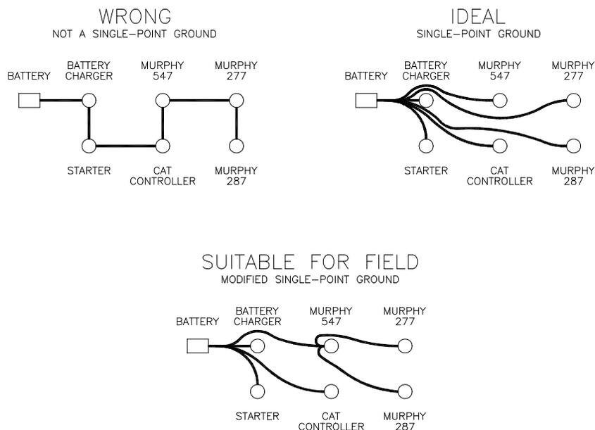
ideal single point signal ground network is one in which separate ground conductors extend from one point on the facility ground to the return side of each of the numerous circuits located throughout a facility. This type of ground network requires an extremely large number of conductors and is not generally economically feasible. In lieu of the ideal network, various degrees of approximation to single-point grounding are employed.
