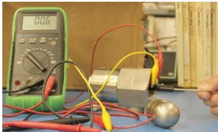
Figure #2 Float is Missing
