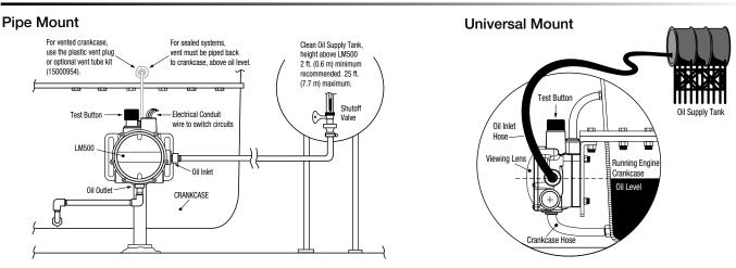
In addition to the direct mounting option, FW Murphy offers two mounting brackets for the LM500. The pipe bracket fits a 7/8 in. (22 mm) diameter pipe. The universal bracket allows various mounting methods. For exact dimensions visit, http://www.fwmurphy.com.
