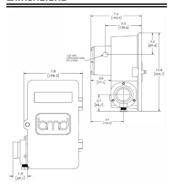
The LC40 measures liquid head pressure, therefore the height above the bottom of the vessel at which the unit is installed is important for the calibration of the unit.
