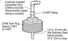
**Tank Plug Kit:** This kit includes 12 ft.  $(3.66 \text{ m}) \times 1/4 \text{ in.}$  (6 mm) diameter stainless steel tube, and fittings for below ground tank installations. The tank plug is available in 2 NPT or 4 NPT and is included with the DLA100 (See "How to Order" on reverse side).
