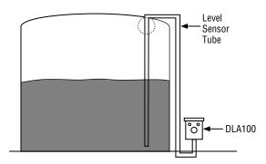
**NOTE**: Tubing for DLA100 must not exceed 150 ft. (45.7 m) from tank for gage to read correctly. Distances greater than 150 ft. require a special quote.
