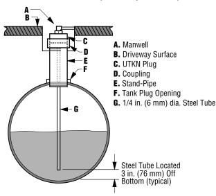
The above method of installation allows for future access should probe tube height adjustments need to be made due to tank settlement, or system troubleshooting.
