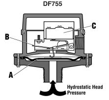
Model DF755 is factory set and operates at approximately 2 in. (51 mm) and 6 in. (152 mm) above the level at which the diaphragm is mounted. The trip point(s) for Model DF757 are adjustable between 2 in. (51 mm) and 110 in. (2794 mm) for high and low (make/break) operation by knobs (D).
