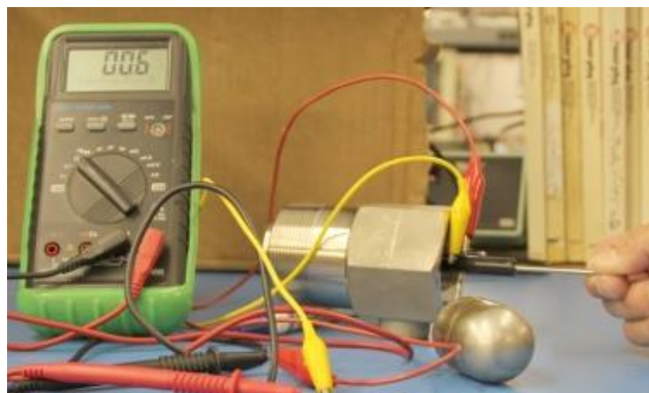
1. Figure #2 Float is Missing
