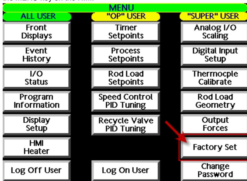
2.13 Next press the Factory Set button on this page. A prompt will appear requiring login using SUPER as the name and the Super user passcode. Refer to the sequence of operation for the panel for proper login credentials.
