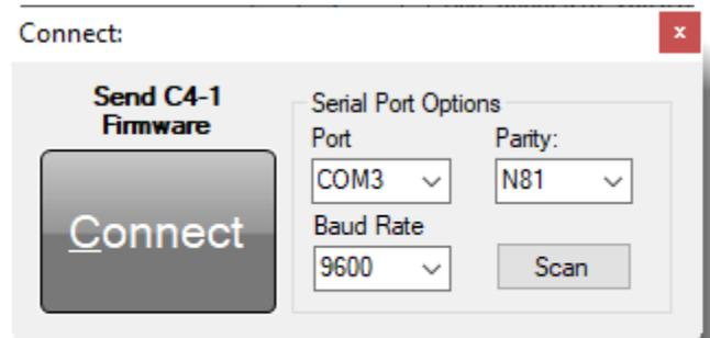
\*If the SCAN button fails to detect the port number, pick the COM port assignment determined by the USB to Serial Bridge manually.
